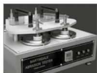
[MARTINDALE TEST] EN16094: 2012 Tested with 320 rotations on the product with a strength of 4N with a scratch pad (Scotch Brite Fleece SB7440).
